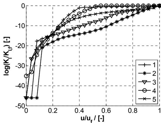
**Figure 3** Liquid transfer coefficient of brick (1), concrete (2), spruce (3), mineralic insulation plaster (4) and plaster (5)
