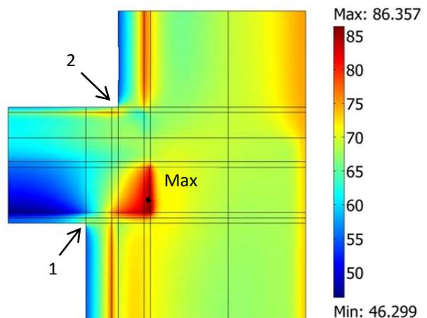
**Figure 9 Water activity distribution on December 31st (case 3, values in %). The yearly evolution at point "Max", "1" and "2" is shown in Figure 10, Figure 11 and Figure 12.**
