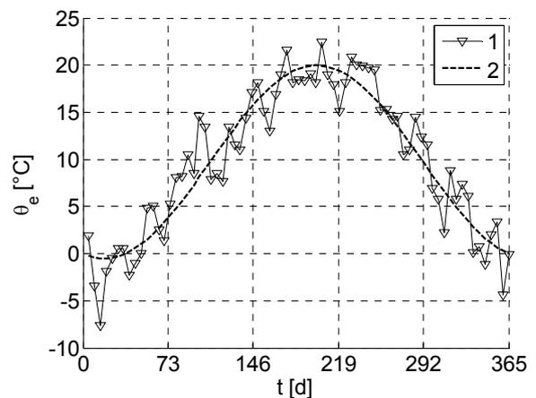
**Figure 6 External temperature. 1: climatic data Innsbruck, METEONORM; 2: periodic approximation**
