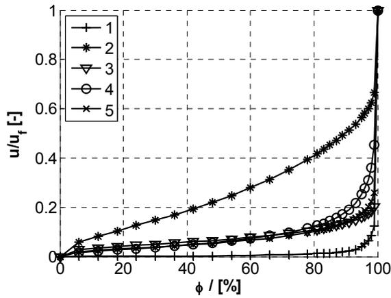
**Figure 1** Water retention curve of brick (1), concrete (2), spruce (3), mineralic insulation plaster (4) and plaster (5)
