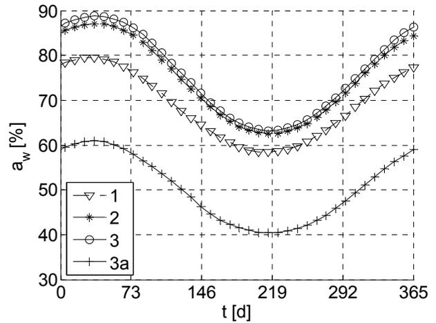
**Figure 10** Temperature and water activity trends at the position presenting maximal water activity (see point Max in Figure 9) for cases 1, 2, 3 and 3a
