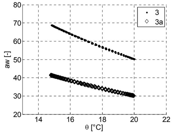
Figure 12 Yearly evolution of water activity versus temperature. Left: lower corner (position 1 in Figure 9). Right: upper corner (position 2 in Figure 9)
