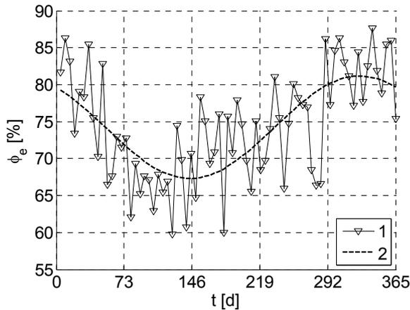
**Figure 7 External relative humidity. 1: climatic data Innsbruck, METEONORM; 2: periodic approximation**
