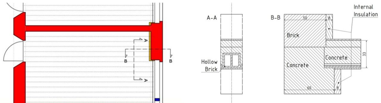
**Figure 4** Floor plan detail (left) and Ceiling-wall section (right), School in Hötting, Innsbruck
