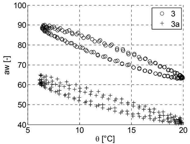
**Figure 11** Yearly evolution of water activity versus temperature at the position with maximal water activity (see point Max in Figure 9) for cases 1, 2, 3 and 3a
