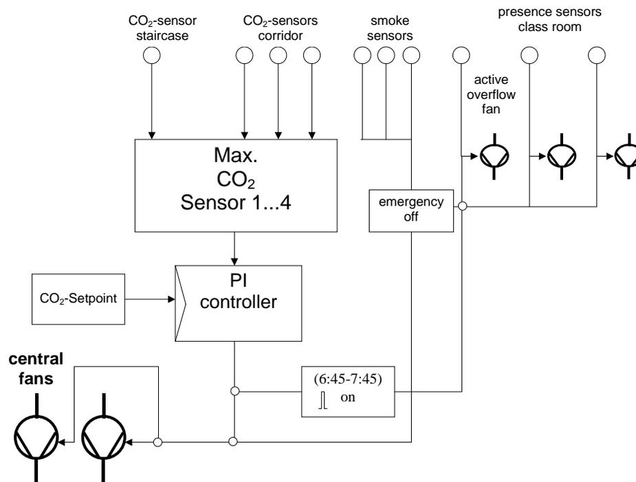
Fig. 4: Control scheme for Central Fans and Active Overflow Fans
