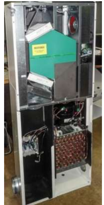
MVHR-unit with micro-heat pump (Project iNSPiRe)
