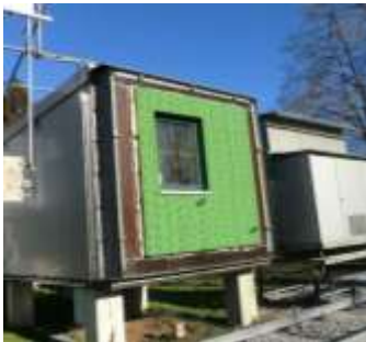
Outside view of wall with integrated micro heat pump (Project iNSPiRe)
