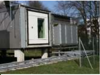
Test cell and Cold-Box in parking position
