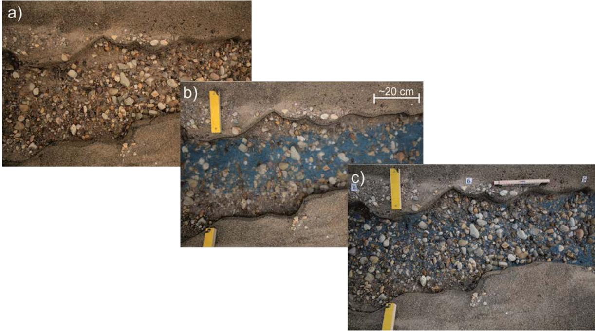
Figure 2: Evolution of the bed surface during an experimental run with a water discharge of 4 litres per second and blue coloured, added sediment: a) initial condition, b) during and c) at the end of the experiment
