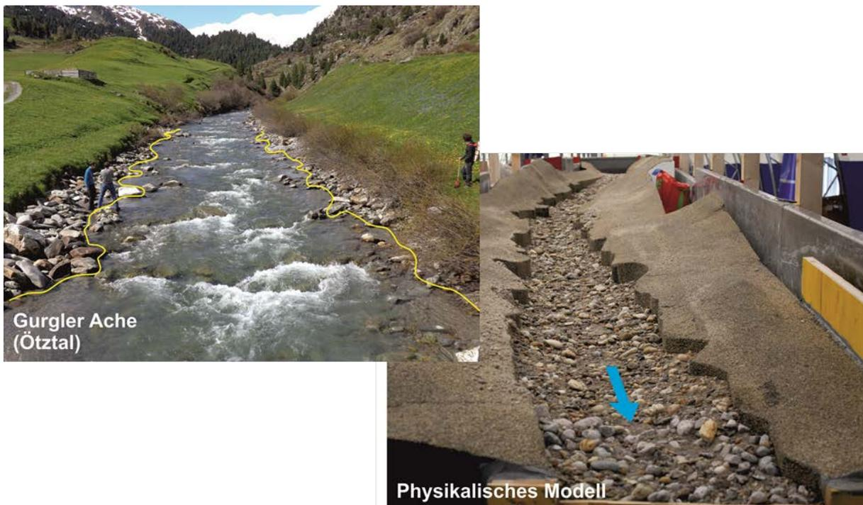
Figure 1: Overview of the prototype reach (left) and the physical scale model (right)
