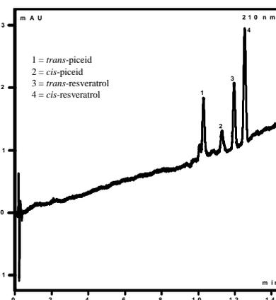
Fig. 3: Capillary: HP-CEC-C18,  $3 \mu\text{m}$ ,  $40 \text{ cm } L_{\text{eff}}$ ,  $100 \mu\text{m I.D.}$ ; buffer:  $10 \text{ mM } \text{NH}_4\text{OAc}$ ,  $50\% \text{ ACN}$ ,  $\text{pH } 6,7$ ; Temp:  $25^\circ\text{C}$ ;  $U = 25 \text{ kV}$ ,  $p = 10 \text{ bar}$ ,  $I = 10,6 \mu\text{A}$
