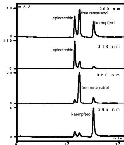
Fig.1: Capillary: HP-CEC-C18,  $3 \mu\text{m}$ ,  $40 \text{ cm } L_{\text{eff}}$ ,  $100 \mu\text{m I.D.}$ ; buffer:  $10 \text{ mM } \text{KH}_2\text{PO}_4$ ,  $60\% \text{ ACN}$ ,  $\text{pH } 7$ ; Temp:  $25^\circ\text{C}$ ;  $U = 25 \text{ kV}$ ,  $p = 10 \text{ bar}$ ,  $I = 12,5 \mu\text{A}$
